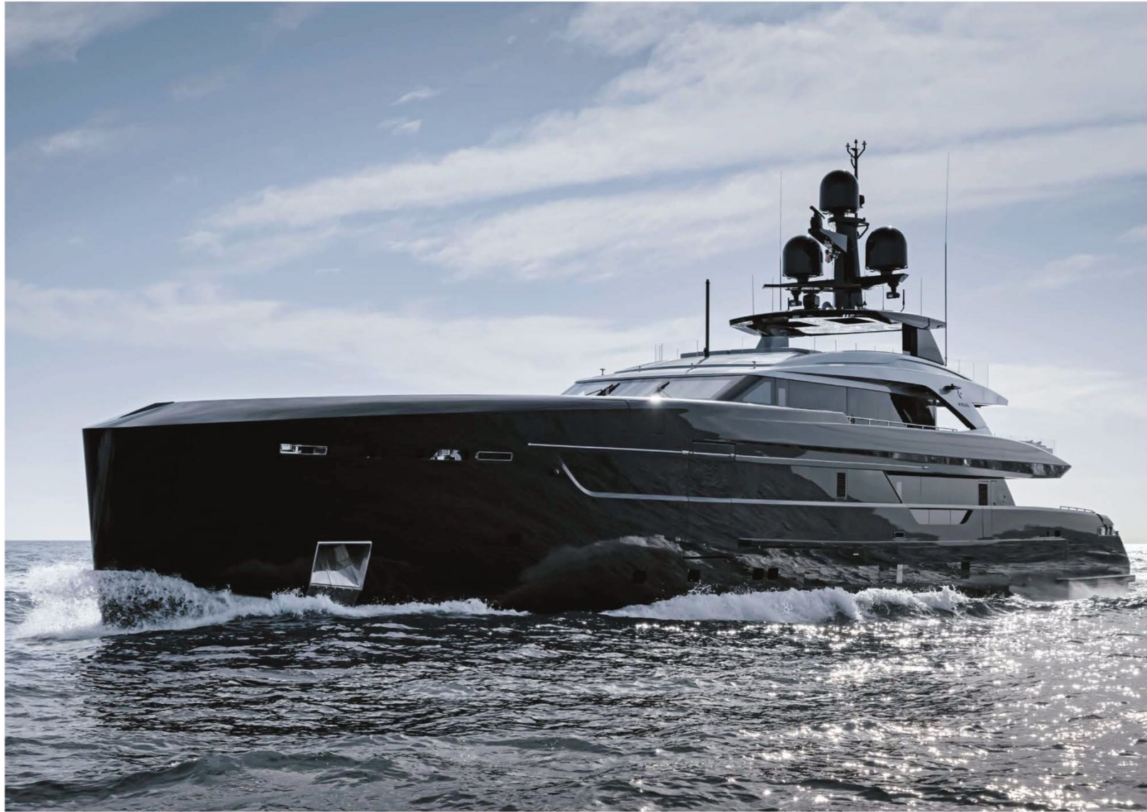
Olokun stands out with her black hull and metallic grey superstructure. Dark hulls can overheat, so Tankoa used the most high-performance coatings available to reduce the temperature of the hull
