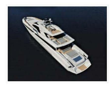
Powered by three MTU engines, providing 2,683hp and combined with the lightweight aluminium alloy construction it is expected the motor yacht will have a top speed of 30 knots and make the yacht their fastest yet.
